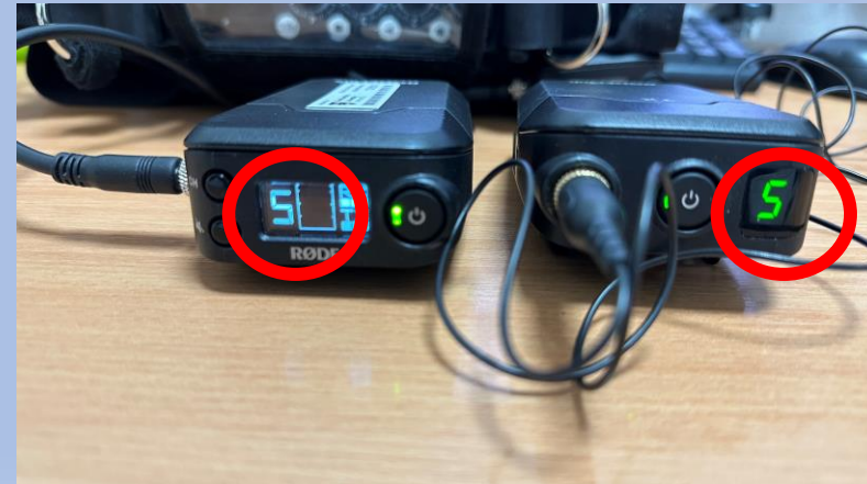
12) The transmitter and receiver will now be paired/matched
