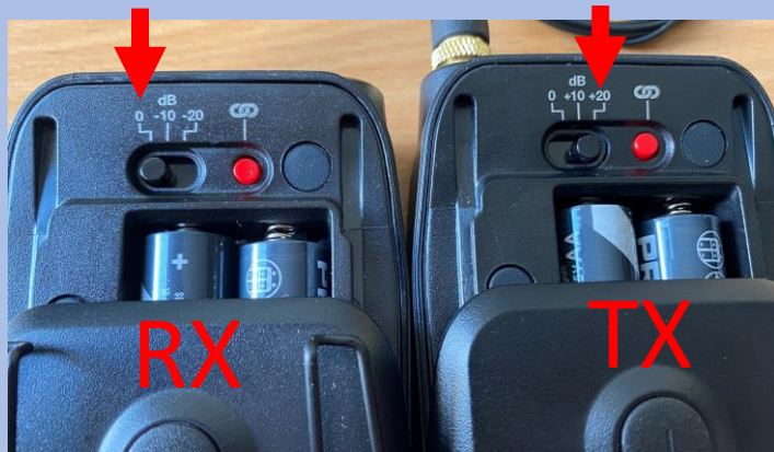
3) ENSURE RX is set to 0 Db and TX is set to +20 Db
